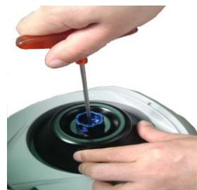
Figure 7: assembling/disassembling the sealed rotor
