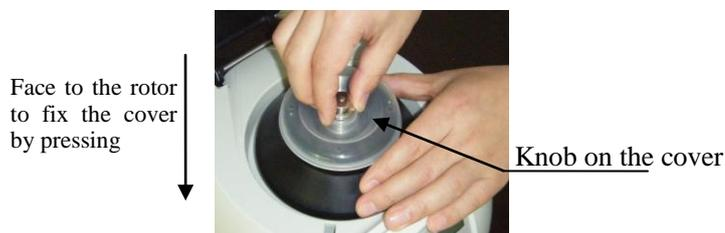
Figure 4: fixing the cover for normal rotor
