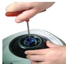
Figure 7: assembling/disassembling the sealed rotor
