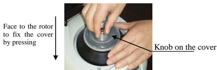
Figure 4: fixing the cover for normal rotor
